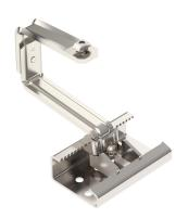
Roof hook to mount photovoltaic modules on pitched roofs in combination with the TP 45 support profile. Suitable for tiled roofs. Screwable fastening on the support profile. Mounting on rafters with TKS wafer-head screws. The roof hook can be adjusted horizontally as well as vertically continuously via glands, correct-Torx 40 key. Height adjustment in the range of the roof slat between 40–54 mm, side adjustment option up to 76 mm, height adjustment of the support profile up to 18 mm
