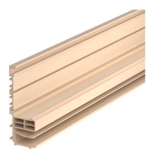
Base of the Rauduo trunking system with 2 individual, thermally separated chambers for joint laying of electrical cables and heating pipes. With locking function for accommodating the trunking covers. The colour of the trunking bases can vary depending on the production method.
